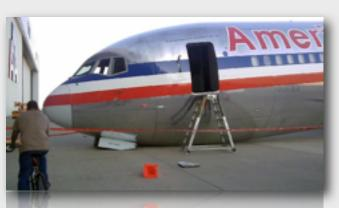
photos show a Boeing 767 on its nose after the front landing gear folded up, dumping the plane onto the ground.
